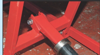
Flip down safety catch, which prevents ram retracting should the hydraulics fail.
