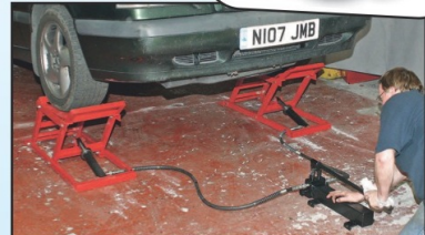
Drive or push the car up them, and pump the ramps to full height.
