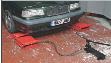
Position the ramps by the tyres of choice (fronts, rears, or both on one side).
