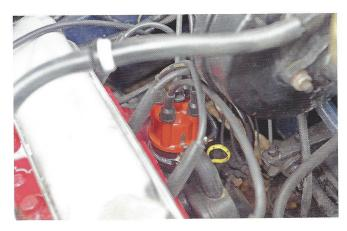
Dispensing with the original points and condenser, and fitting an electronic ignition instead, is one of the easiest ways of improving reliability.
