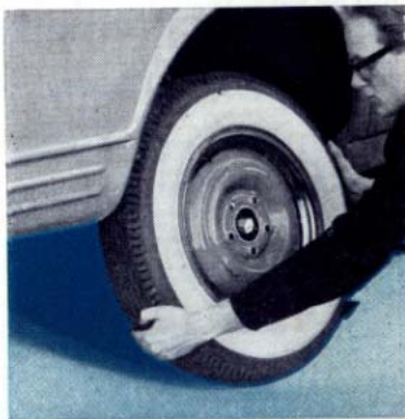
4. Screw off the wheel nuts and lift off the wheel. Fit on the spare wheel and tighten the nuts a little at a time, taking alternate nuts. Do not tighten up the nuts excessively as otherwise the wheel disc and threads may get damaged.
