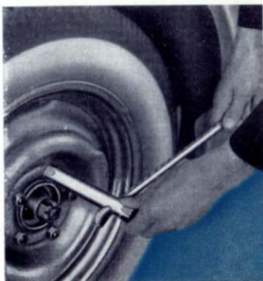
2. Slightly slacken all five wheel nuts with the same tool.
