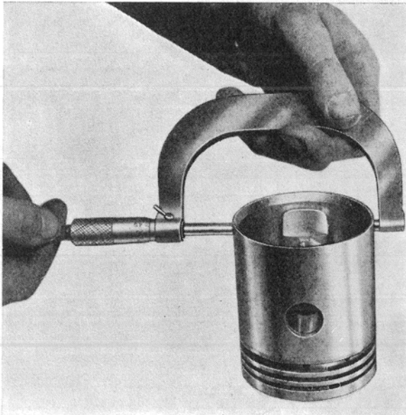
Fig. 35. Measuring a piston.
