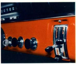
illuminated for night driving. An unusual detail here is that the heater supply system is thermostat controlled. This means that the temperature maintained remains at exactly the level adjusted and is practically independent of driving conditions and weather.
