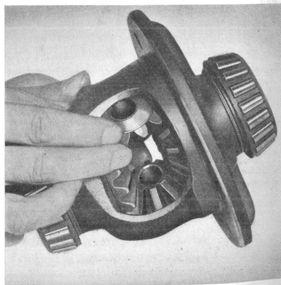
Fig. 29. Assembling the differential gears.
