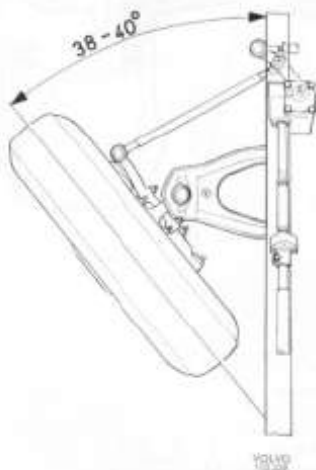
Fig. 6-10. Adjusting max. wheel lock
