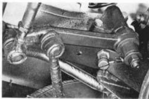
Fig. 6-11. Adjusting screw, max. wheel lock 1. Adjusting screw
