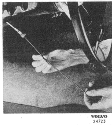
Fig. 28. Lubricating the drive cable
