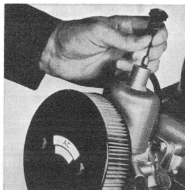
Fig. 2. Checking oil level in centre spindle
