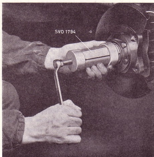
Fig. 18. Removing the inner bearing.
