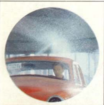
Rigid check — water test
