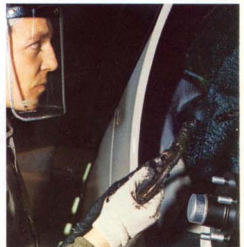
Comprehensive underbody sealing before the cars leave the factory
