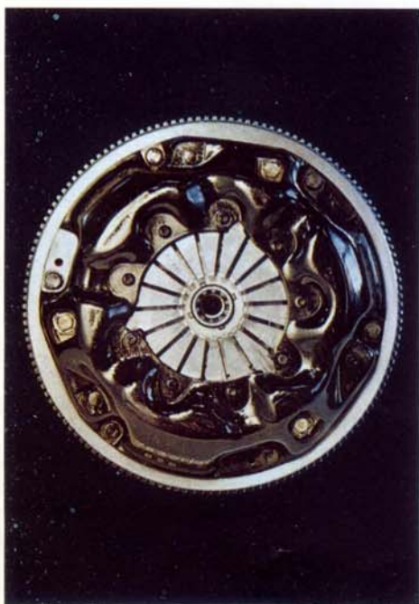
The diaphragm clutch requires less pedal pressure
