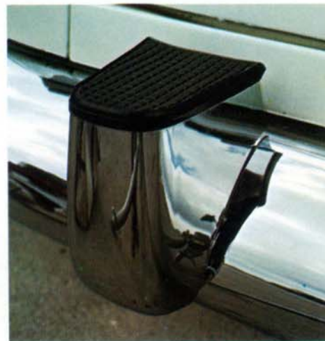
The rear bumper guard acts as a step up to the roof rack.
