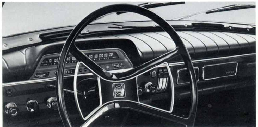
The steering wheel is especially designed to absorb impact.
