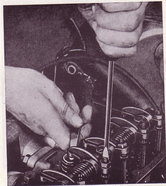
Fig. 28. Adjusting the valve clearance
