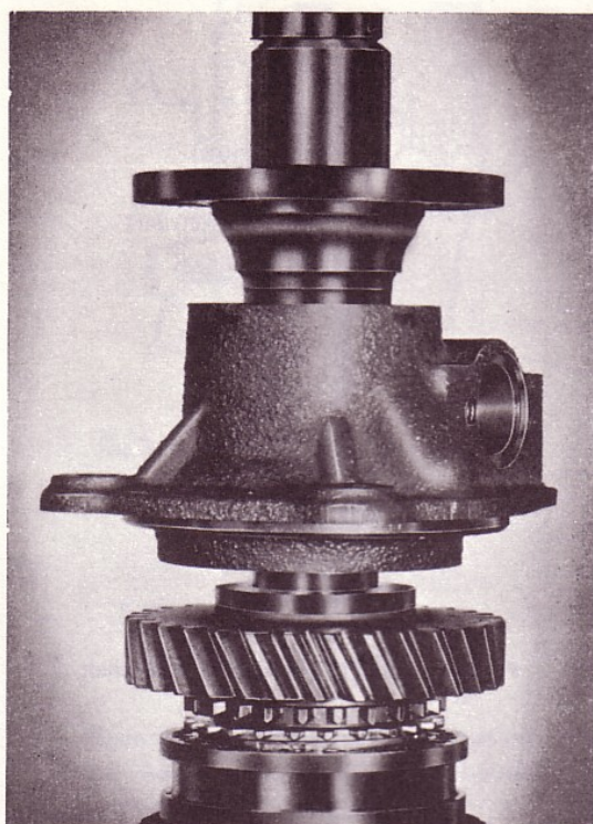
Fig. 26. Fitting rear cover, M 40
