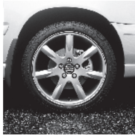
Volans 7 Spoke 7"x17" S70, V70, 850 (94-) 9451521-0 Tire Non AWD 205/45 ZR17 88W PZero, AWD 215/45 ZR17 91W P6000
