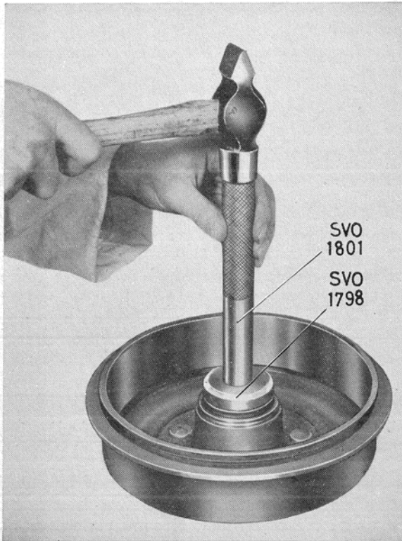
Fig. 19. Fitting sealing ring.
