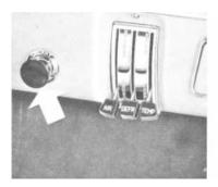
Switch for fresh-air fan Pushed right in - closed Interco. pos. - full output Fully out - half output
