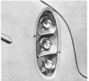
is the flasher, the middle one the combined stop/tail light, and the bottom one the back-up light. See that the glass seats properly on the gasket when assembling the fixture. The untinted part of the glass should be at the bottom.
