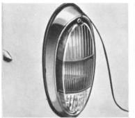
Unscrew the two screws, one at the lower end of the lighting fixture, by means of a Philips screwdriver and lift off the glass and the metal frame. The bulbs can now be removed by pushing in and twisting anti-clockwise. The top bulb
