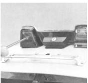
The number plate lighting is built into the handle on the luggage compartment lid with one bulb on each side of the emblem. The bulbs are accessible from the underside of the emblem.
