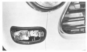
The larger one is the flasher and the smaller one the parking light. See that the glass seats properly on the gasket.
