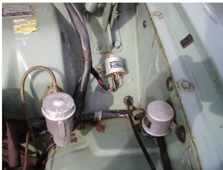
Relay placement in engine bay
