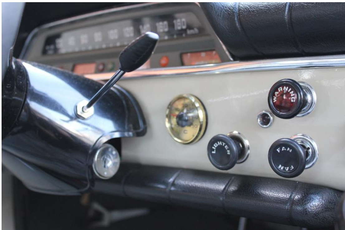
Overdrive switch on steering wheel column and control lamp on instrument panel
