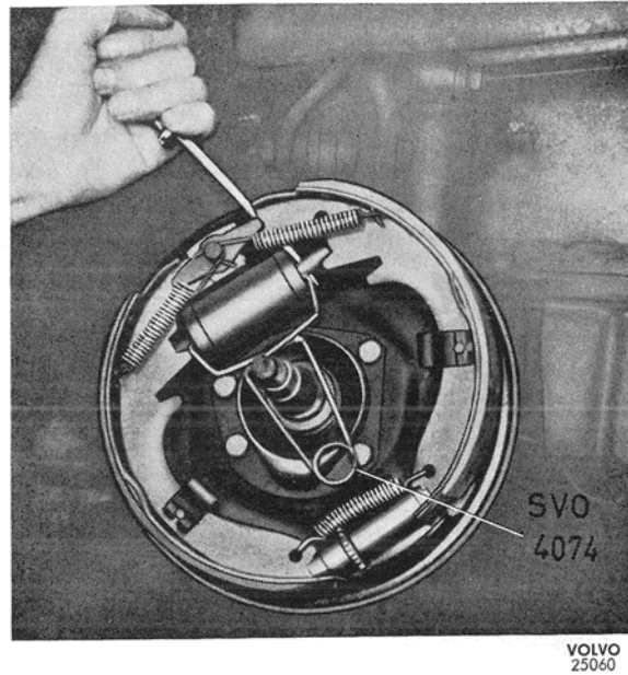
Fig. 24. Removing the wheel unit cylinder
